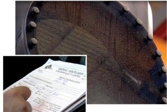
Water leak test
